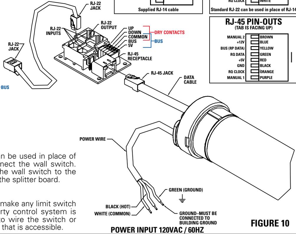
3-conductor 20-24 gauge wire can be used in place of the supplied RJ-14 cable to connect the wall switch. Connect the BUS terminals on the wall switch to the corresponding BUS terminals on the splitter board.
