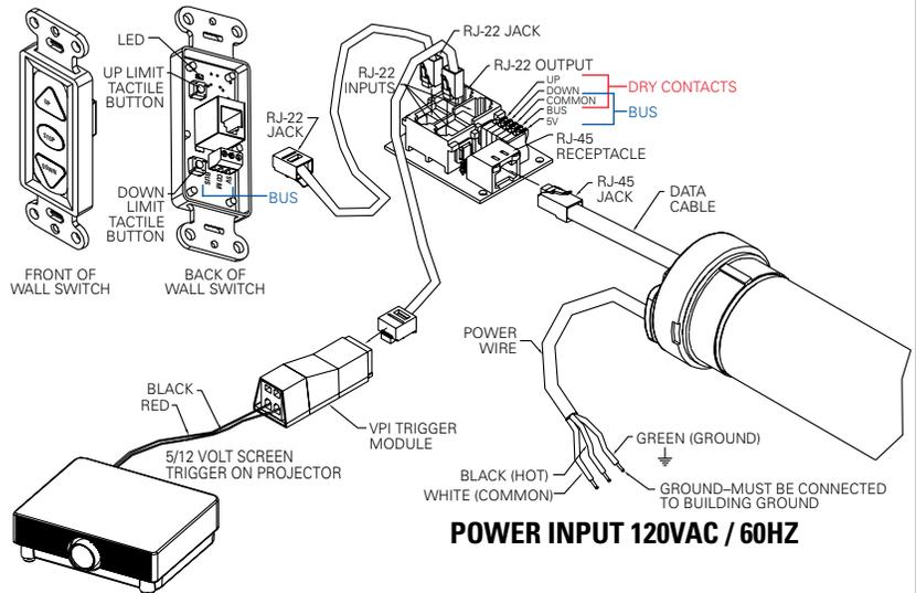
**240V WIRING DIAGRAM WITH OPTIONAL BUILT-IN VIDEO PROJECTOR INTERFACE**
